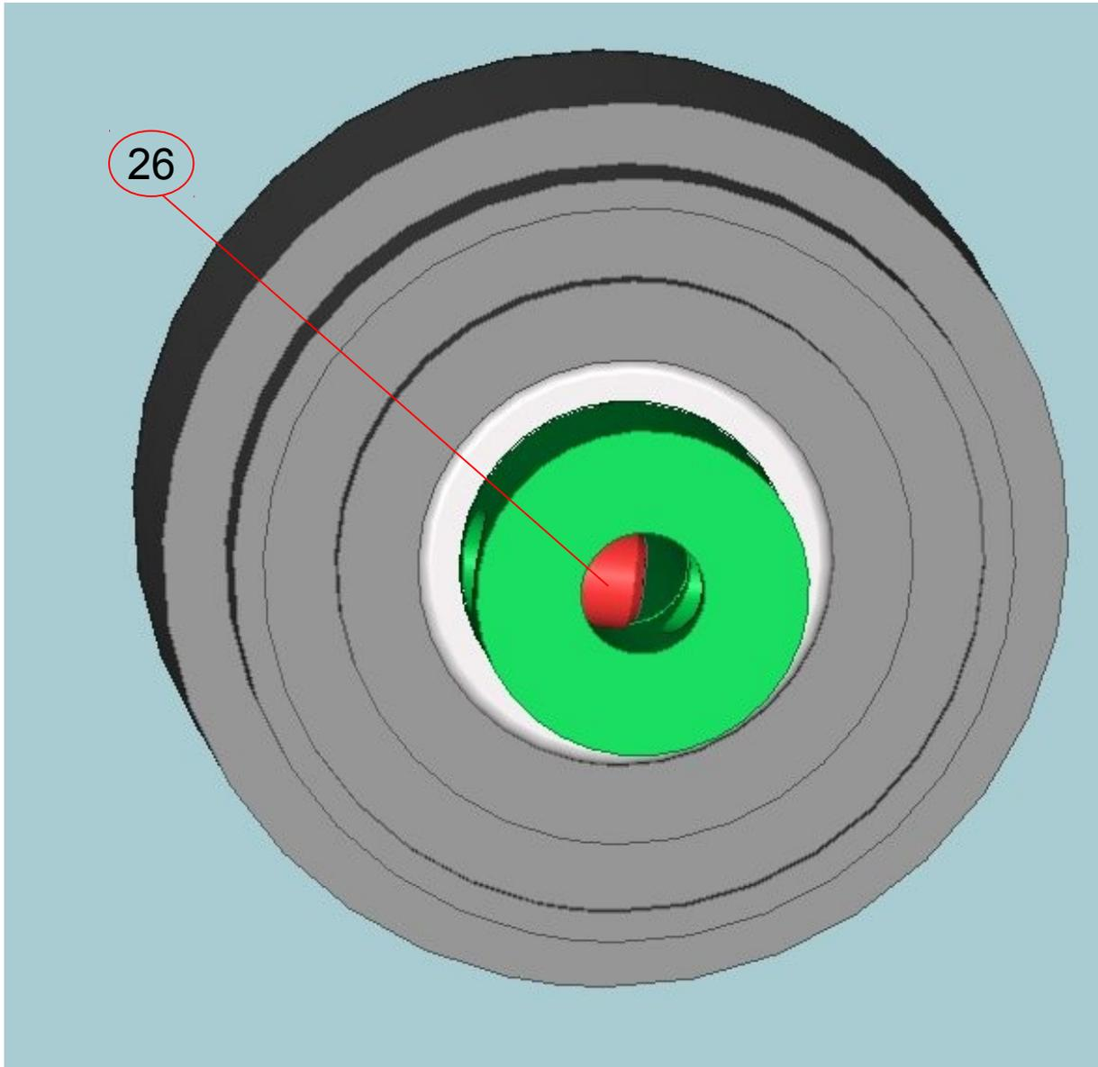
6) Insert mini screw in the front wheel hub all the way, until it's completely inside the aluminium hub
