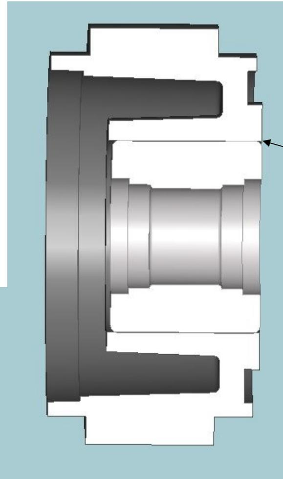
**Bearing must be aligned in the plastic wheel so that its inside surface is aligned with the inside surface of the plastic wheel.**
