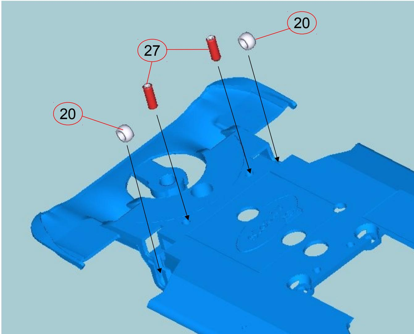
16) turn chassis upside down, and insert two 6mm mini screws in the special holes. Also add two bushings in the front axle supports.
