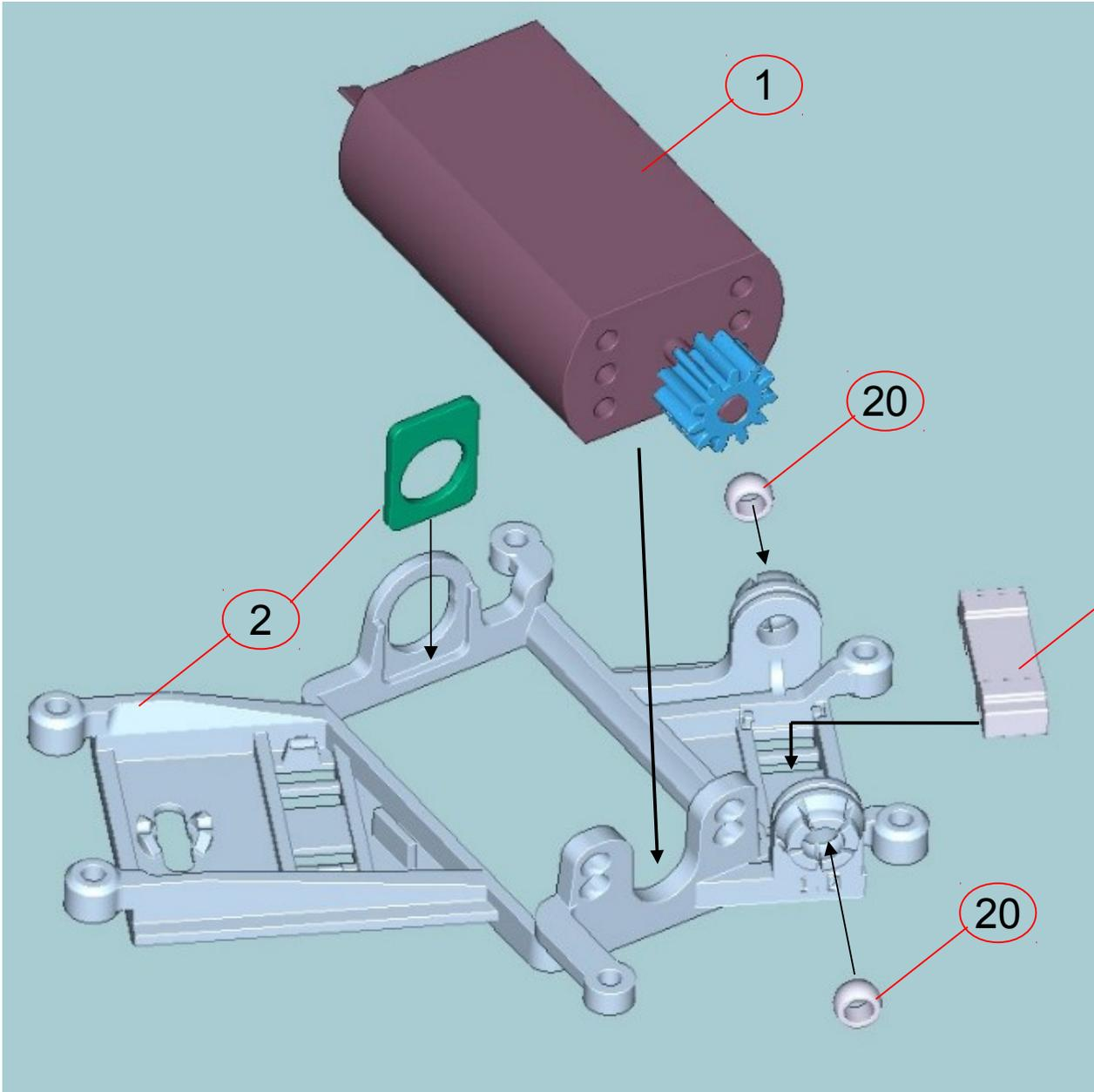
14) Add standard motor mount parts: motor, magnet, bushings, adapter
