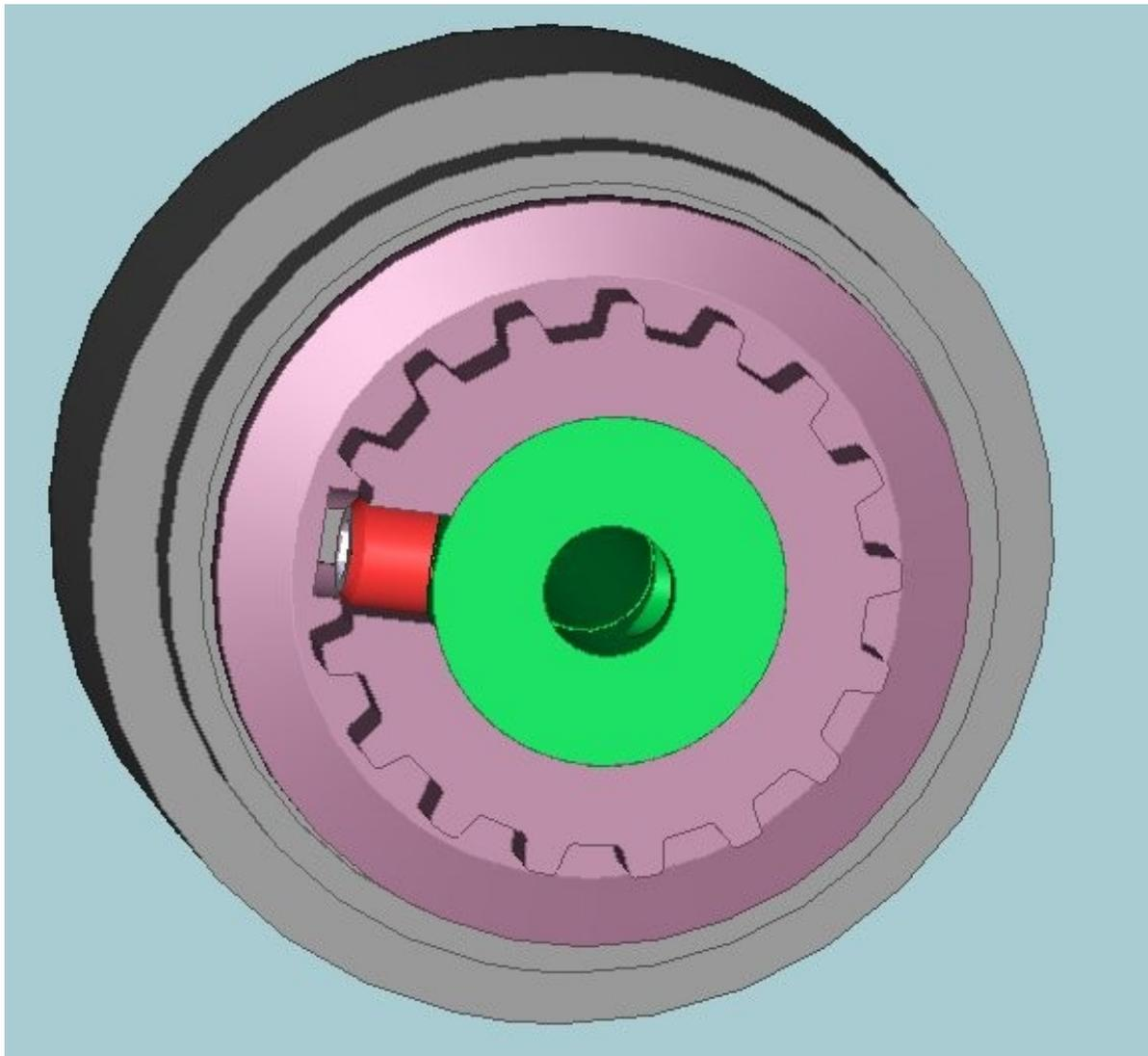
8) Unscrew the miniscrew so that the axle can be inserted in the front wheel.
