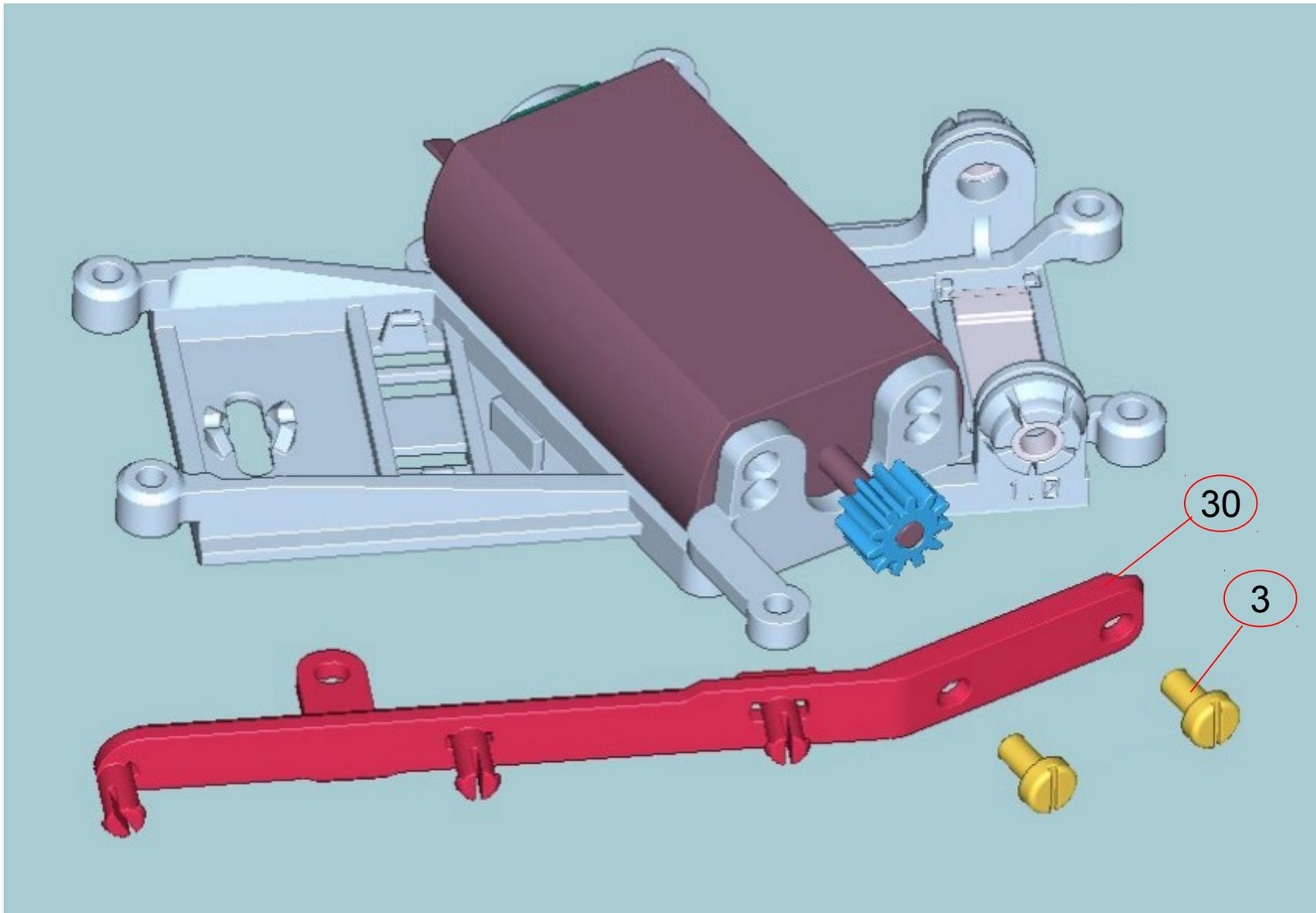
15) Screw the motor to the motor mount, keeping the pulley tensioner between the motor mount and the heads of the screws
