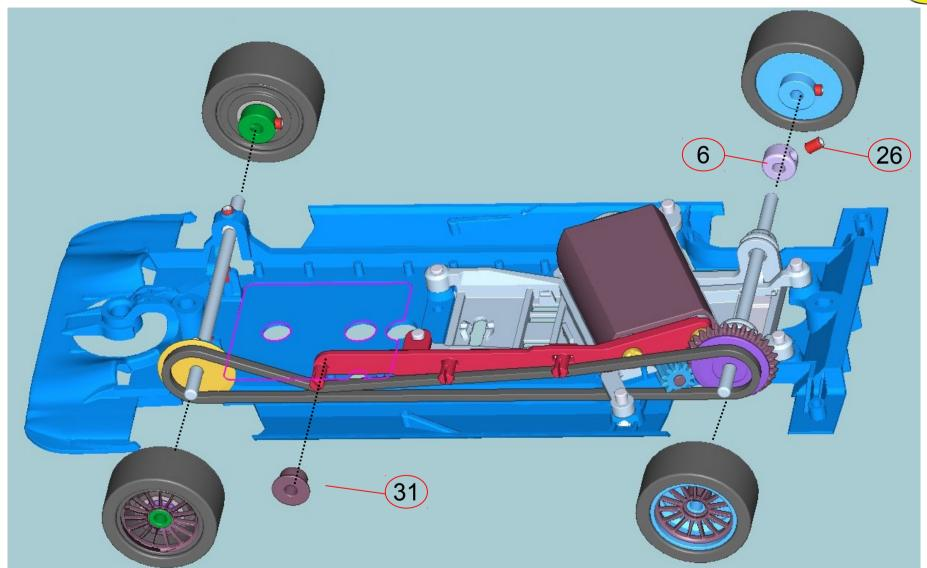
22) insert the flanged plastic bearing on the tensioner. Add the RIGHT wheel and the LEFT wheel. Add rear stopper and right wheel, with mini screws. Now assemble the left wheels, making sure the belt is in the proper place on the pulleys!!
