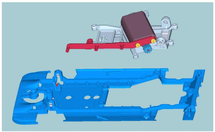
18) add motor mount assembly (use 2 body type screws at front of the motor mount, and 4 standard motor mount screws for the rest - side and rear. See image in next slide)
