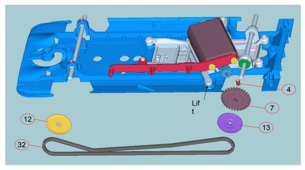
20) insert yellow Z28 crown with mini screw. Add front 0.3 flange spacer and rear 0.7mm flange spacer Lift the left side motor mount screw post and insert the toothed belt
