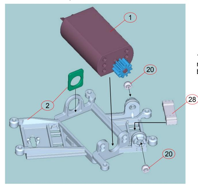
14) Add standard motor mount parts: motor, magnet, bushings, adapter
