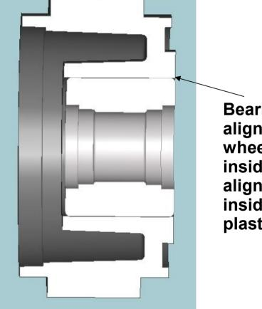
Bearing must be aligned in the plastic wheel so that its inside surface is aligned with the inside surface of the plastic wheel.
