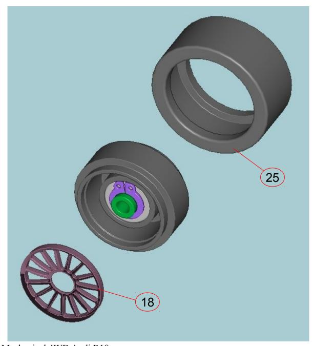
4 - Mount front wheel insert and tyre
