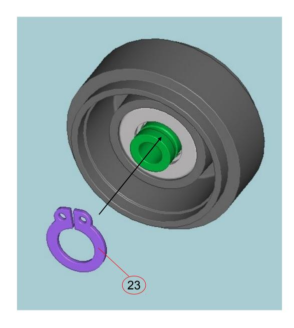
3 - Use the special seeger ring pliers to mount the seeger ring in the recessed guide, to assemble bearing and aluminium hub together.
