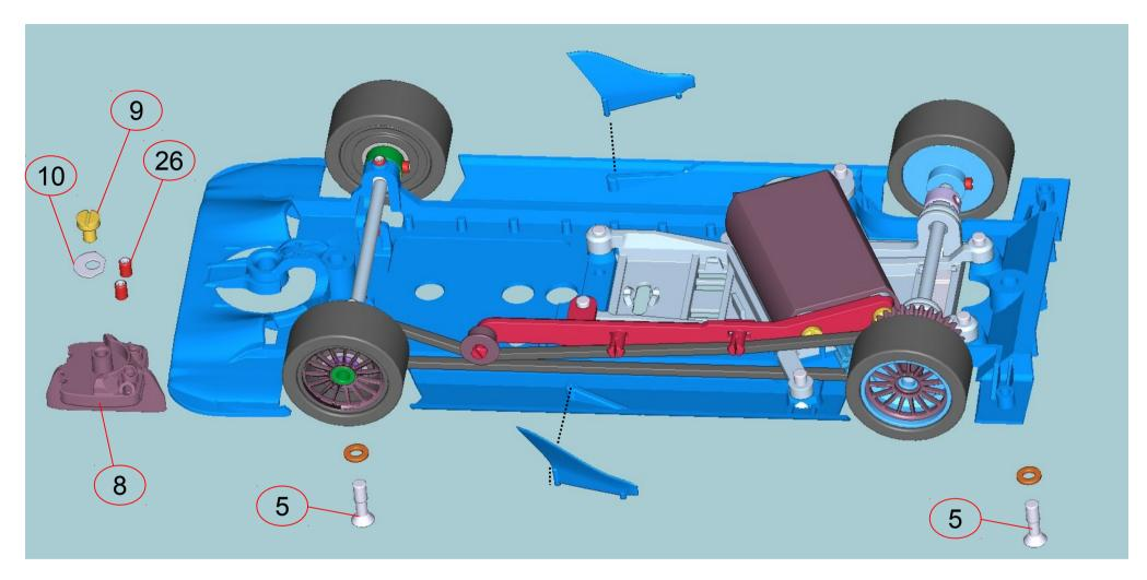
23) add pickup, side fins, and assemble to body.
