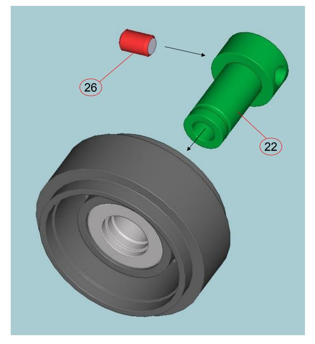
2 - Insert aluminium hub in the bearing, and insert the mini screw M2x3 in one of the two hub holes
