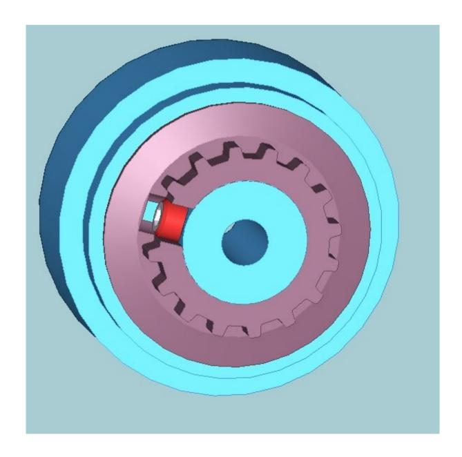
12) Unscrew the miniscrew so that the axle can be inserted in the rear wheel
