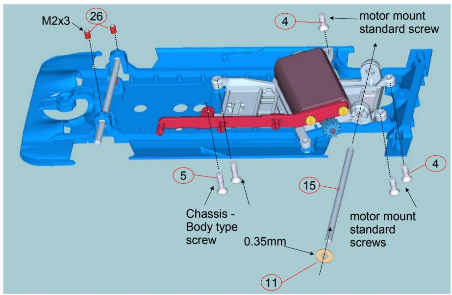
19) add 2 mini screws 3mm on the top of the front shaft, and insert 0.35mm rear spacer
