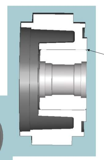
Bearing must be aligned in the plastic wheel so that its inside surface is aligned with the inside surface of the plastic wheel.
